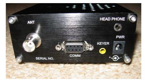
The power jack is a standard  $5.5 \times 2.1$  mm jack coaxial power jack. The center pin is the positive connection, and the outer shell is the negative connection. Connect the radio to a suitable power source of 9.6 to 14.5 volts, direct current.
