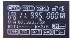
**TS+:** Frequency Step up. Underline shows digit that can be changed. **MD:** Mode for LSB-USB-CW.
