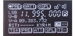
**PRE:** Turn the preamplifier on or off. **ATT:** Select the input attenuator. Not implemented on this model. **SPL:** Run in "split" mode.
